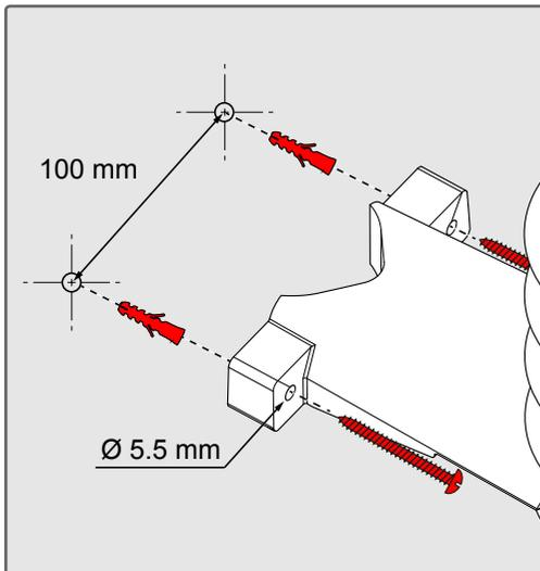
**Mount the transmitter on a wall using suitable screws and wall plugs (not included).**
