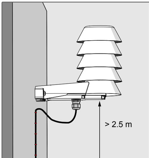
**Install at least 2.5 m above ground. Avoid placing transmitter near ventilation, windows, and heat sources.**
